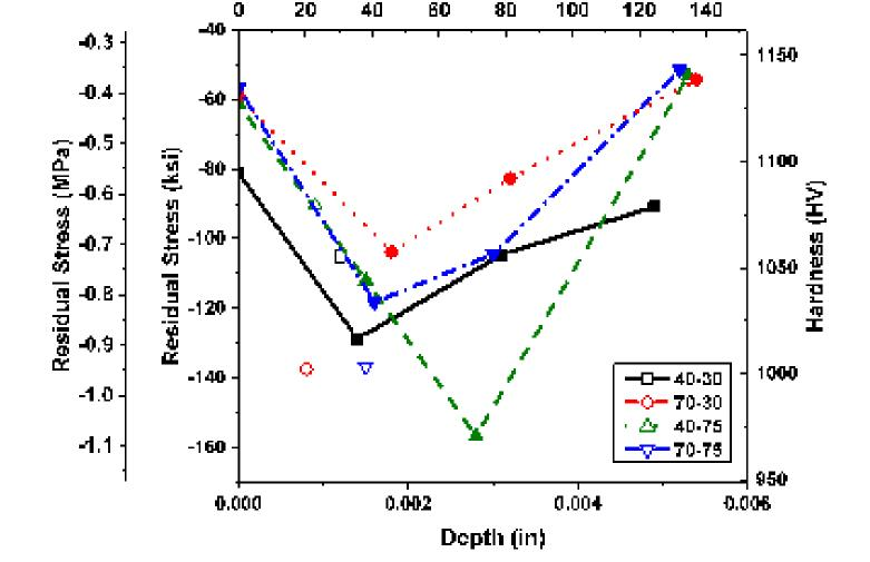
The residual stress profiles and the maximum hardness value and location for the four experimental samples. 40-75 shows the greatest residual stress at the deepest location, along with the highest hardness value.
