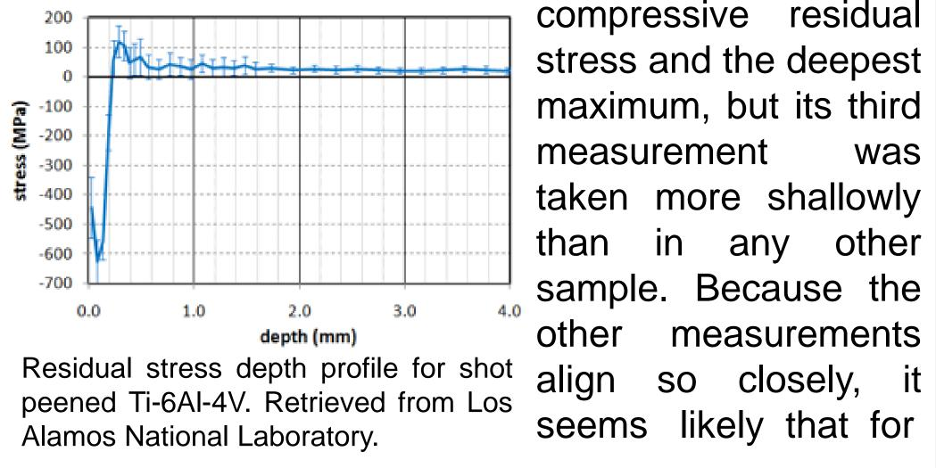
the other three samples, the true peak compressive residual stress was missed as it occurred between the second and third measurement depths.
