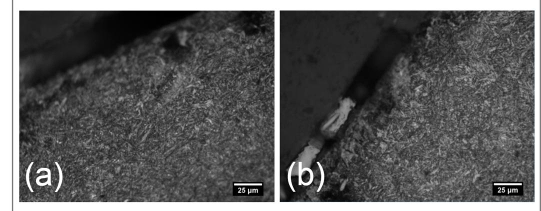
Image (a) shows the microstructure near the surface of the peened region for 40-30. Image (b) shows the same region for 40-75. All samples had microstructures comprised of tempered lath martensite. Small, semi-circular, white areas reveal the presence of cementite, more heavily present in Image (a) than in Image (b).
